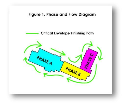
After analyzing the project schedule, it appears there may be an area for improvement when it comes to the sequence that the façade is installed. A potential solution to the schedule would be starting on a more critical corner of the building where site constraints may cause delays further in
